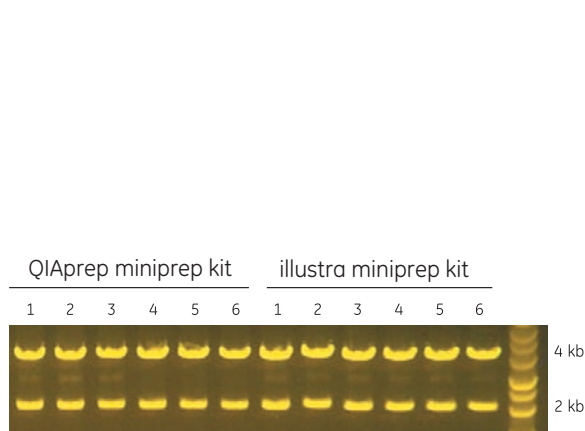
Fig 3. HindIII restriction digests (1 unit, 37°C for 1 h) of plasmid DNA samples. A representative image is shown of plasmid DNA samples extracted from culture 1.
